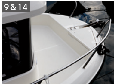
Foredeck anchor locker and stainless steel tilt bow roller with optional forward windlass Bow area suitable for fishing
