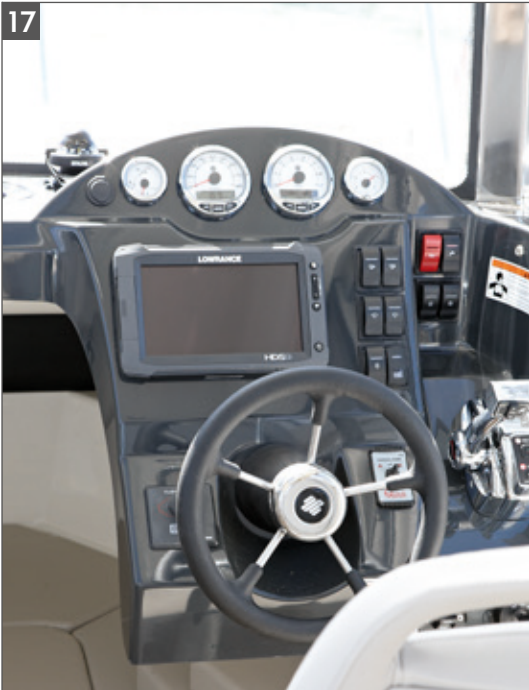
Integrated helm with hydraulic steering, SmartCraft instrumentation, mounting area for optional 9" GPS/Chart plotter/Stereo
