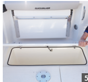
2 fish lockers with standard drains and optional port electric pumpout available with Fish Pack
