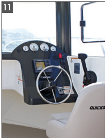
Integrated helm with hydraulic steering, mounting area for optional 7" GPS/Chart plotter/Stereo and 12v outlet
