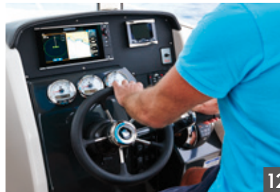
Helm with hydraulic steering, SmartCraft, optional 9" GPS/Chart plotter, Fusion radio and 12v outlet
